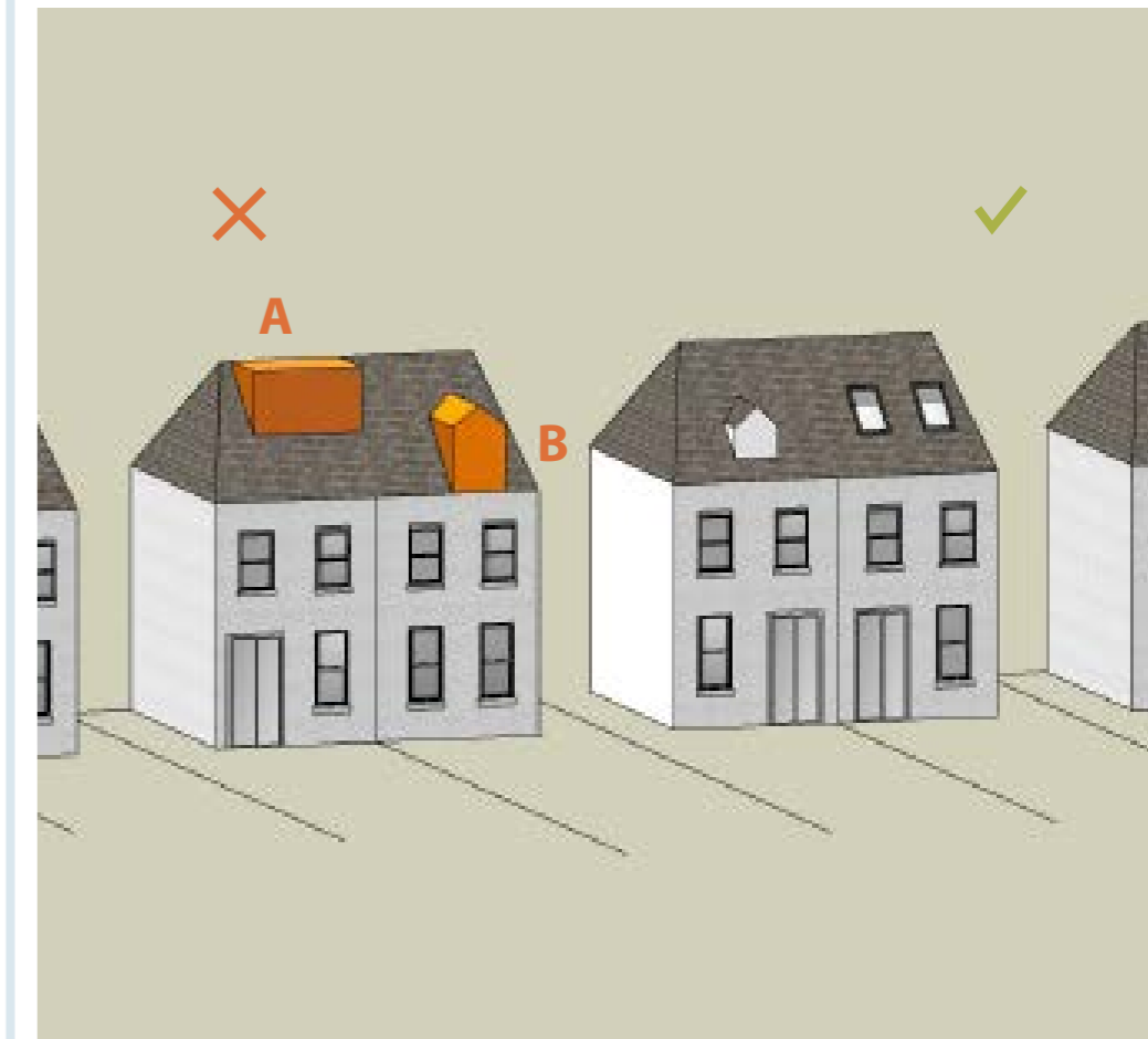
A - Dormer roof extension sits on the ridge line and is both out of proportion with existing windows and overbearing on the property as a whole.
